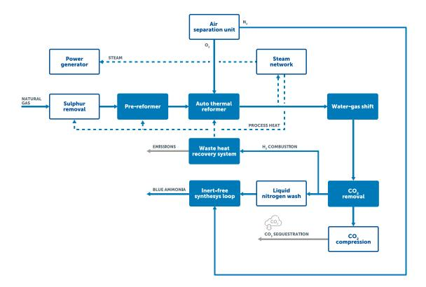
**Ammonia Synthesis** - After adding with  $N_2$ , the purified, inert-free syngas is compressed and directed to a Casale ammonia synthesis loop, equipped with a Casale Axial-Radial® ammonia converter, where low-carbon, cold ammonia is produced. The high efficiency of the converter and the reactivity of the inert-free gas ensure that equipment sizes in the synthesis loop and refrigeration section are within the limit of industrially proven references.
