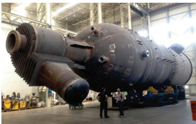
**Figure 4.** Oxygen blown ATR for 7000 tpd methanol plant.
