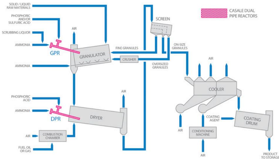
**Figure 1.** Dual pipe reactors process block diagram.
