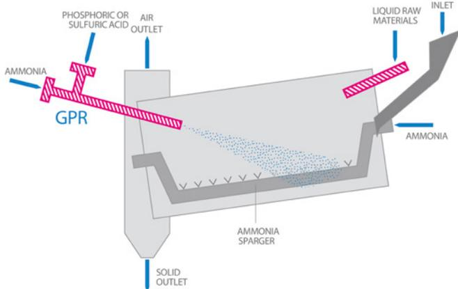
**Figure 2.** Drum granulator with granulator pipe reactor (GPR).
