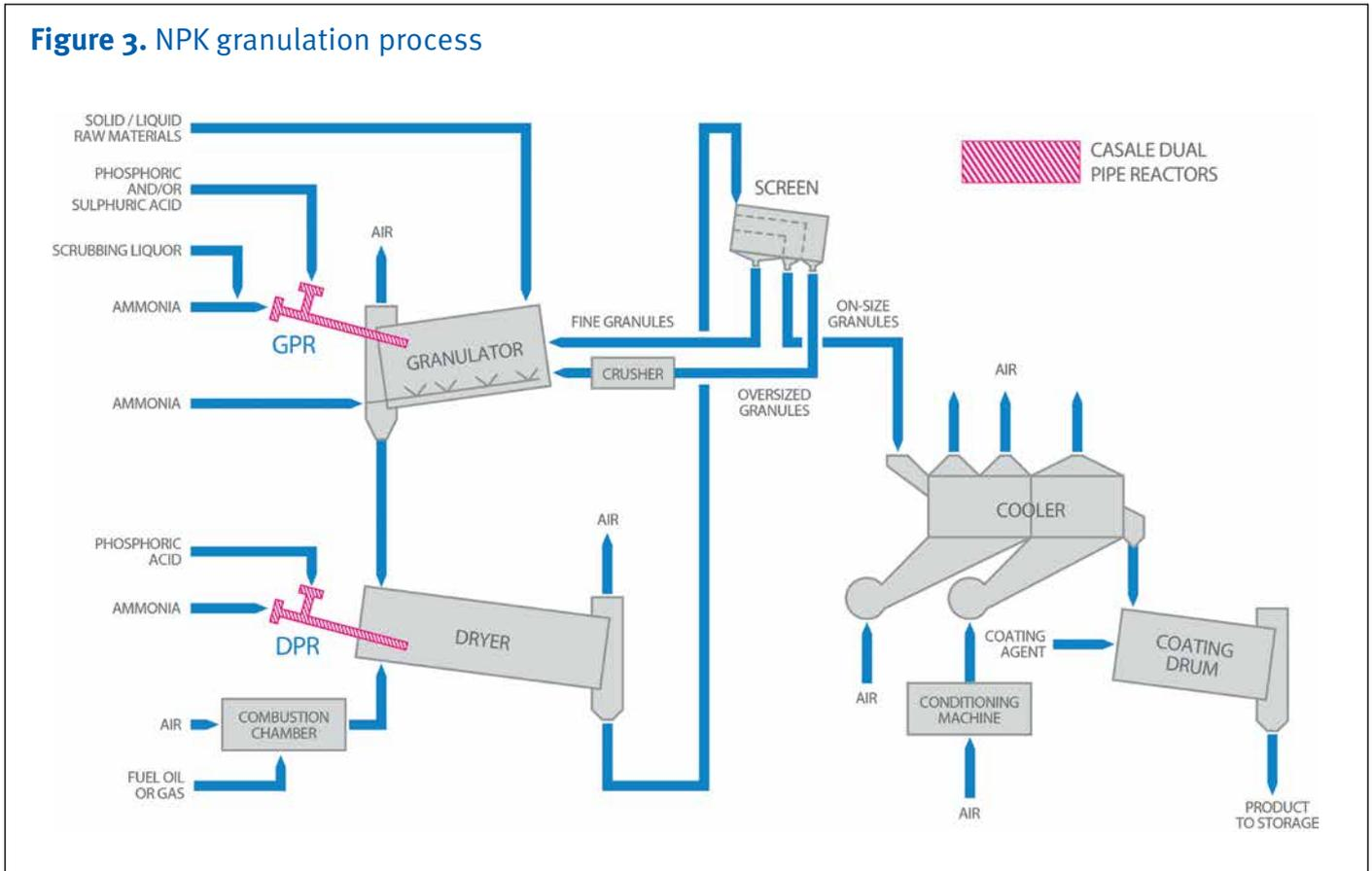
Casale’s granulation process for NPK production is described below. It is based on phosphoric acid and potassium chloride as raw materials for P and K respectively, while the N source used can be ammonia with either ammonium nitrate or urea.
