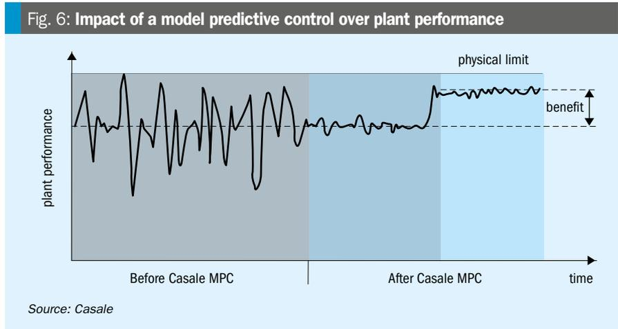
the software allows the efficiency of the urea synthesis to be maximised by dynamically targeting the optimum N/C, H/C and operating pressure in the urea reactor. This is possible thanks to the power of the physical process model which supports the MPC operation by suggesting the optimum value of the critical controlled variables depending on the real plant capabilities and constraints.
